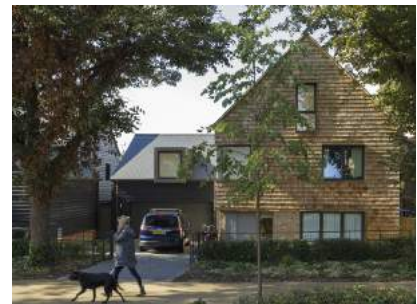
CAR PARKING ON-PLOT AT SIDE OF HOUSE AND BEHIND BUILDING LINE. THE AVENUE, SAFFRON WALDEN
